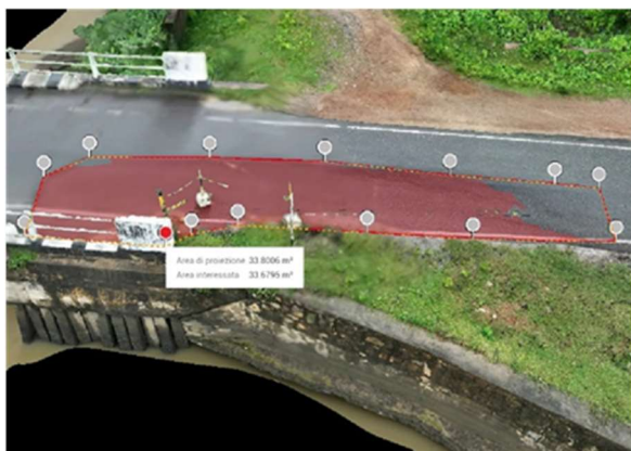
Photo 7 Mesh 3d area measurement – Photo 8 Dem (.tif)
