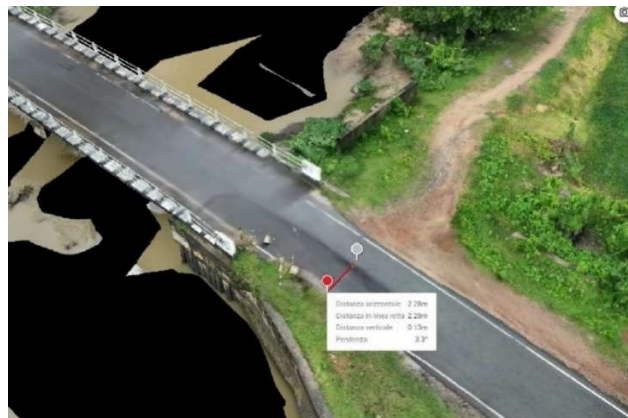
Photo 3 – Damage in proximity of the abutment (left) - 3D-modelling throw drone survey and assessment of the damaged area (right)
