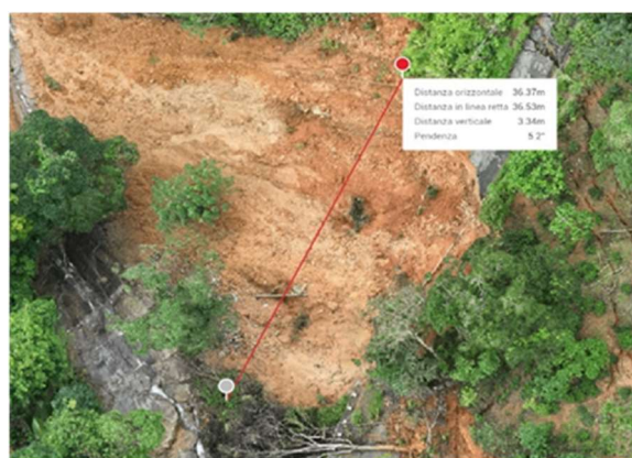
Photo 3 ortofoto (.tif/.geotiff) – Photo 4 ortofoto (.tif/.geotiff) linear and aerial measurement
