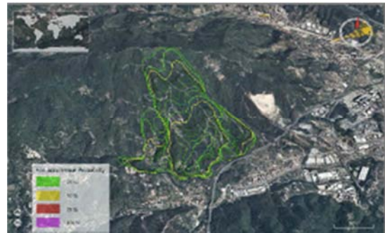
Figure 6.12 - Propagator. Final 75% fire probability hourly isochronous lines
